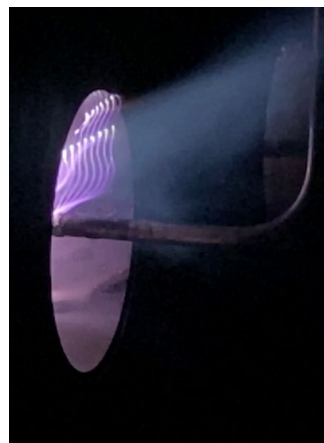
Photograph of elongated spark discharges in the BIMER-PAC burner
