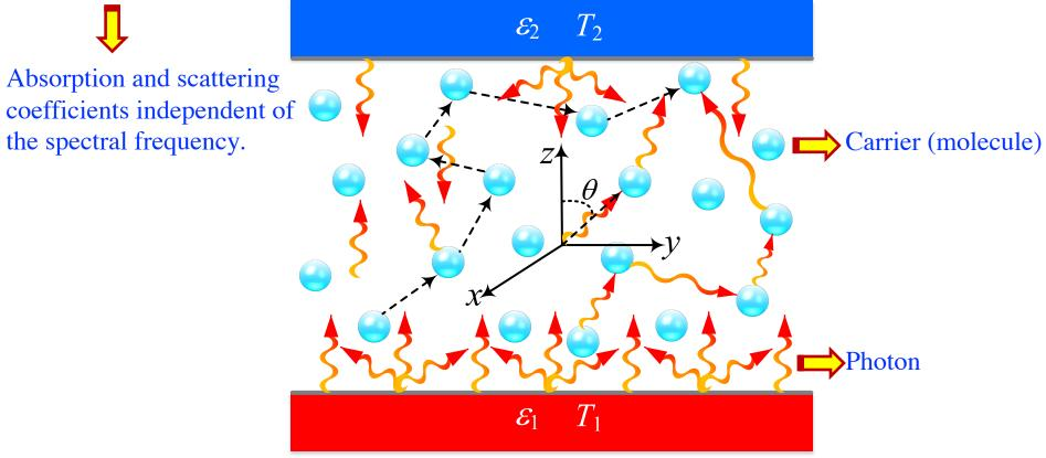
Heat transfer by **photons** as well as by **photon-carrier** and **carrier-carrier** interactions
